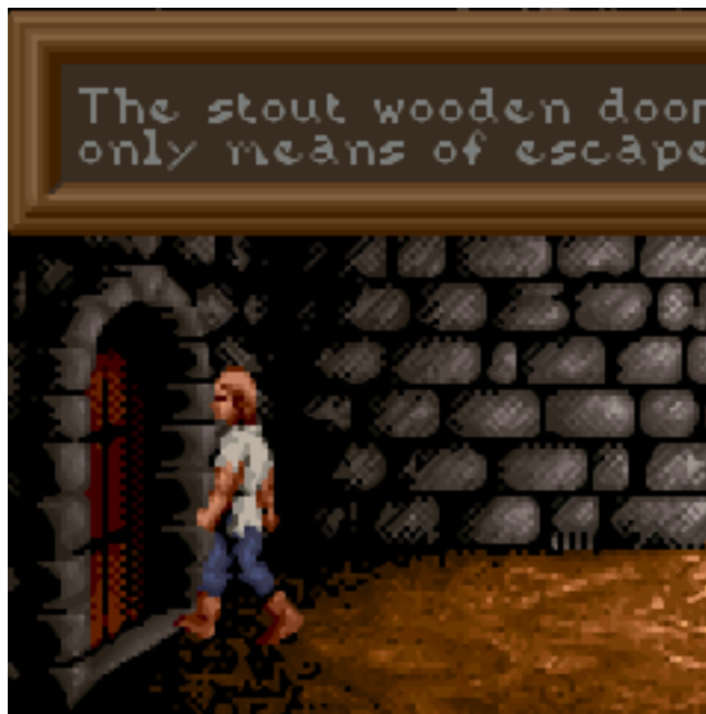
Fig. 15: PM 2x : Analyzes the eight neighboring pixels to create smoother diagonal lines and rounded edges.
