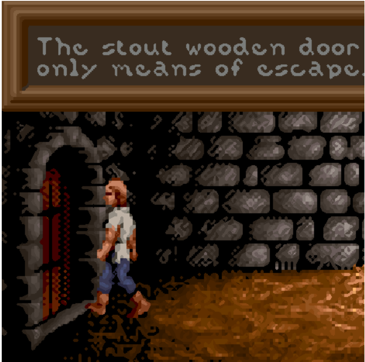
Fig. 11: AdvMAME 3x : Expands each pixel into 4 new pixels based on the surrounding pixels. Doesn't rely on blurring like 2xSAI, fast.
