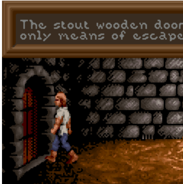
Fig. 9: AdvMAME 2x : Expands each pixel into 4 new pixels based on the surrounding pixels. Doesn't rely on blurring like 2xSAI, fast.
